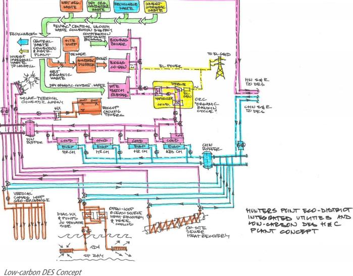
future "6th Generation Multi-Energy Systems," which aim for the flexibility to include a multitude of energy sources and end-use forms including multiple energy conversion technologies, thermal (heating and cooling) and electrical distribution networks, and thermal and electrical storage.
